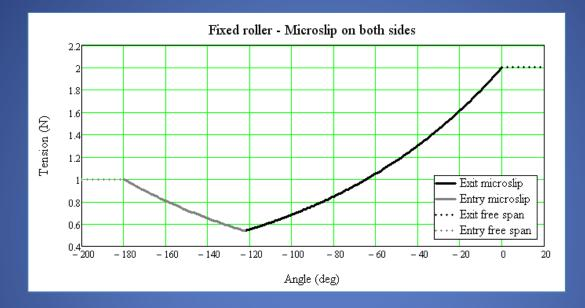
It should be mentioned that this isn't the only possible microslip geometry. If the difference in the weights is reduced, a point will be reached where a constant tension zone develops between the two curves. If the difference in the weights is increased, a point is reached where one of the microslip zones consumes all of the wrap angle and the belt will slip off the roller.
