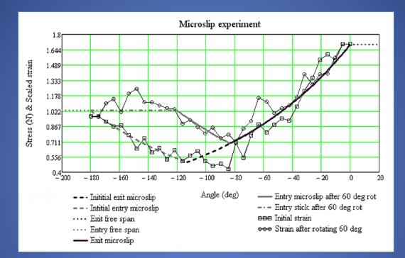
It's apparent that a considerable amount of stick-slip remained. The data shown here was smoothed using a running average with a coefficient of 0.5. Significant Poisson contraction was evident and may also have affected the assumption of uniaxial stress. However, everything considered, the data fits surprisingly well. It's good enough to provide at least modest assurance that the reasoning is correct.
