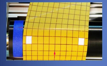
Microslip can be present without any net transfer of torque to a roller.
