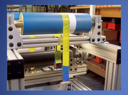
The scale marks on the latex were 1/10 inch (2.54 mm) apart. Since they were made by hand using a metal scale, it was calibrated while relaxed and flat on a table, using a precision scale and a magnifying glass.
