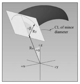
Figure 5 - A Section of a Torus
