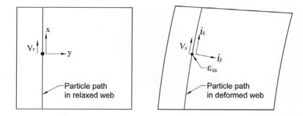
Figure 2 - Geometric relationships in the Velocity-Strain equation
