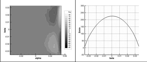
Figure 8-Shear stress, elliptic web Axes in radians, stress in psi
