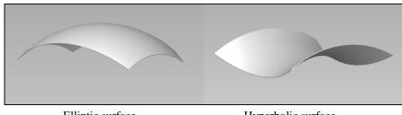
Elliptic surface Hyperbolic surface Figure 4 – Two fundamentally different curvatures for baggy webs
