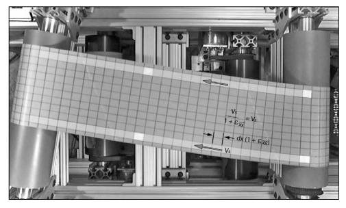
Figure 3 Qualitative Demonstration of the Velocity-Strain equation.
