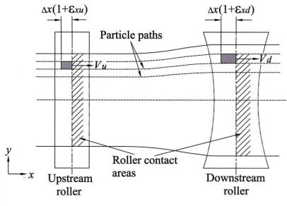
Figure 4 The normal strain rule
