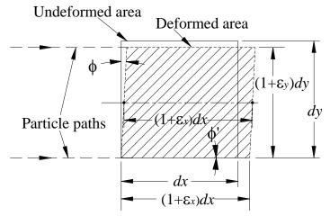
Figure 5 Effect of shear on the normal strain rule
