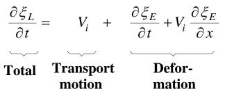
The second step is to apply the Euler description to the deformation term. Subscripts are now used to identify the displacement variable as either Lagrange (L) or Euler (E).
