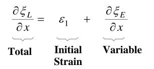
To be consistent, the strain will also be separated into two parts - a constant component that exists at time zero when the only particle velocity is the transport motion, plus a component due to the disturbance.
