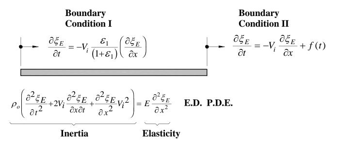
Applying the Euler description to the one-dimensional wave equation and to the boundary conditions produces the model above. The P.D.E. is the wave equation for a moving medium. It appeared in one of the earliest traveling string papers. In that instance it applied to out-of-plane motion.
