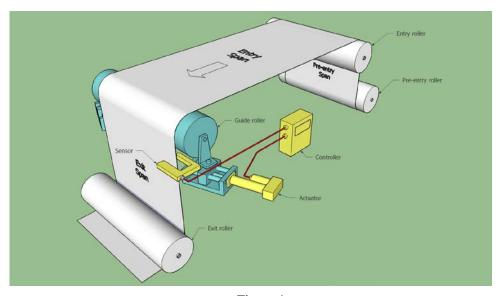
Figure 1 A typical web guiding system Remote pivot type (also known as a steering guide)
