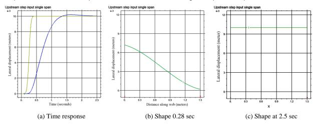
Response between fixed parallel rollers due to a change in upstream position
