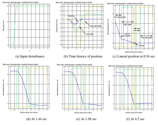
**Figure 8** Response to a step input at 0.54, 1.41, 1.98 and 4.5 seconds
