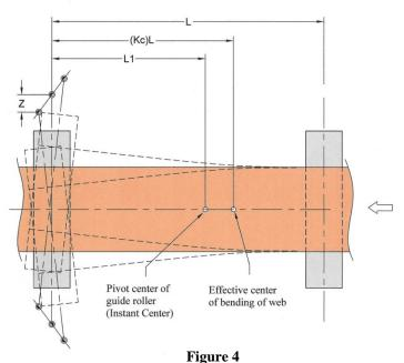
Web curvature (steady state response to roller misalignment)
