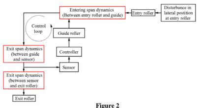
Block diagram of steering guide of Figure 1
