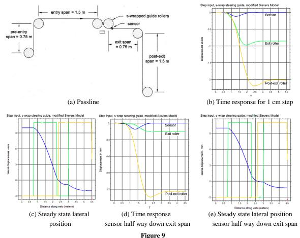
Step response of system with exit span in the same plane as the entry
