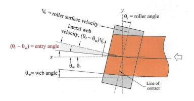
Figure 3 Entry angle (function of both roller angle and web angle)
