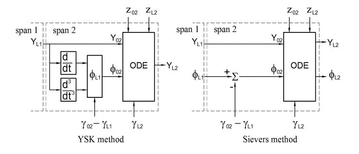
In the YSK method, only the lateral displacement is passed to the next span. Since all of the information about its derivatives is implicit in the lateral displacement, it is possible to reconstruct the cross section rotation from the previous span by mathematical manipulation.
