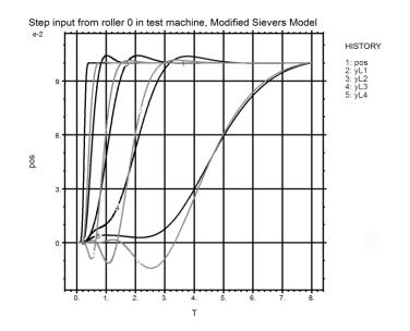
The four spans have lengths of 10, 22, 40 and 120 inches. Curves show the lateral displacements at the downstream ends of each one. The dark lines are for the Timoshenko model and the gray lines are for the Euler Bernoulli model. The leftmost curve is the input displacement at the upstream roller of the first span.
