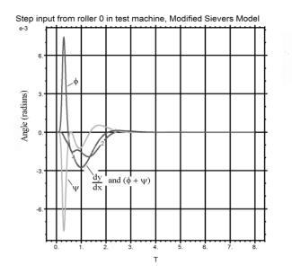
This graph shows  $\phi$ ,  $\psi$  and  $dy_L/dx$  for the downstream end of the second span. The sum of  $\phi$  and  $\psi$  is also plotted, but isn't visible because it is identical to the curve for  $dy_L/dx$  (as it should be). It is clear that for this span,  $\phi$ ,  $\psi$  and  $dy_L/dx$  are comparable to one another in magnitude.
